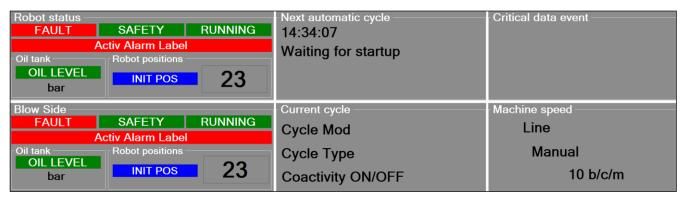
The remote display, located near the forming machine, allows operators to easily monitor the status of the FlexRobots when working around the forming machine.
